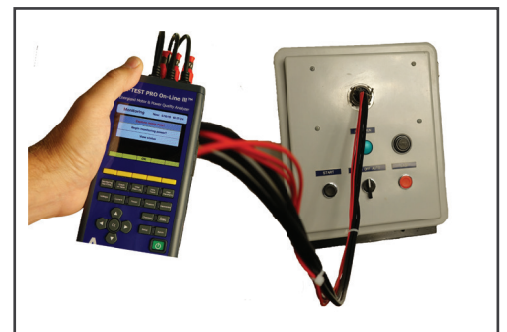
Installed ALL-SAFE inside starter box, connected to ATPOL III™ to start taking readings.
